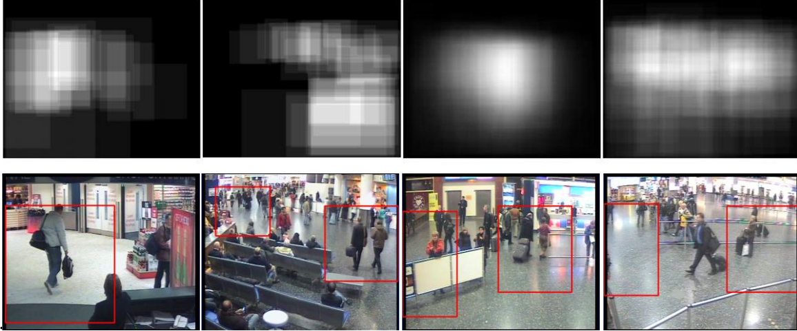
Figure 2. the probability maps of the 4 different scenes (the first row)and the predefined regions (the second row)
