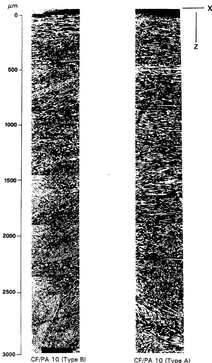
Figure 10. Micrograph sections showing the fibre orientations for **STATIC** and **DYNAMIC** processes in PA/c composites. These sections are in the z-x plane at the centre of the moulded plaque.
