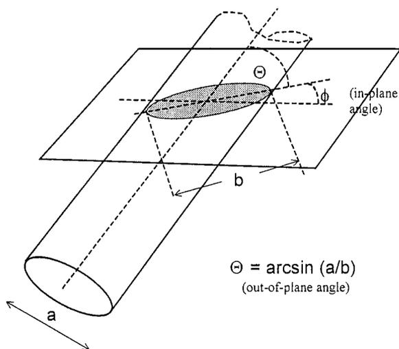
Figure 7. Description of the in-plane and out-of-plane angles.
