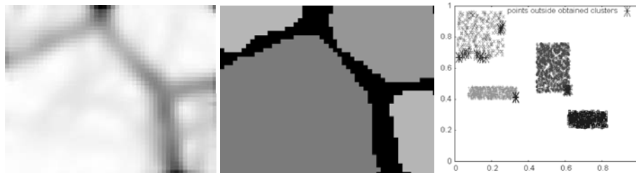
Figure 2: Visualization of the typical "mean distance to neighbors" matrix for the SOM obtained on the 2D data set of fig.1 (left). Corresponding segmentation of the SOM produced by our algorithm (middle). Clustering result (right): no points are affected to the wrong cluster, and only a few "border" points end up unclassified (big stars).
