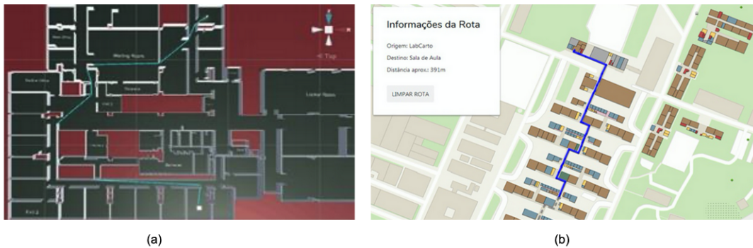
Figure 4.3: Automatic generation of indoor tactile maps: (a) 3D map was generated from an AutoCAD floor plan described in [81], and (b) map was generated from the indoor-routing schema described in [13]
