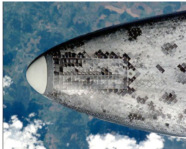
Ceramic tiles on space shuttle
