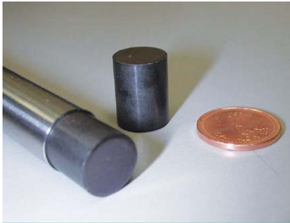
\text{UO}_2 ceramic pellet
