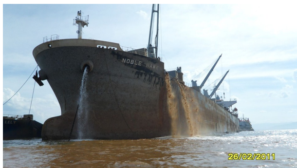
Figure 1: Handymax bulk carrier NOBLE HAWK aground on an uncharted pinnacle in E. Indonesia 2010.
