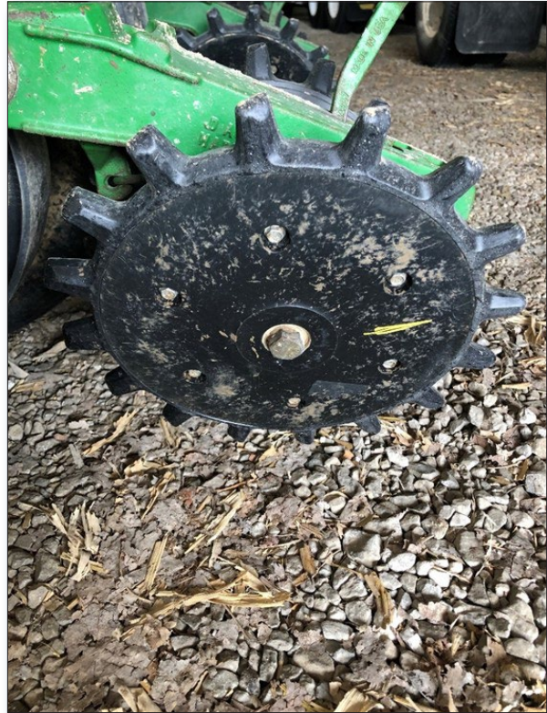
Figure 2. Closing wheel equipment modification for no-till corn and soybean planting.
