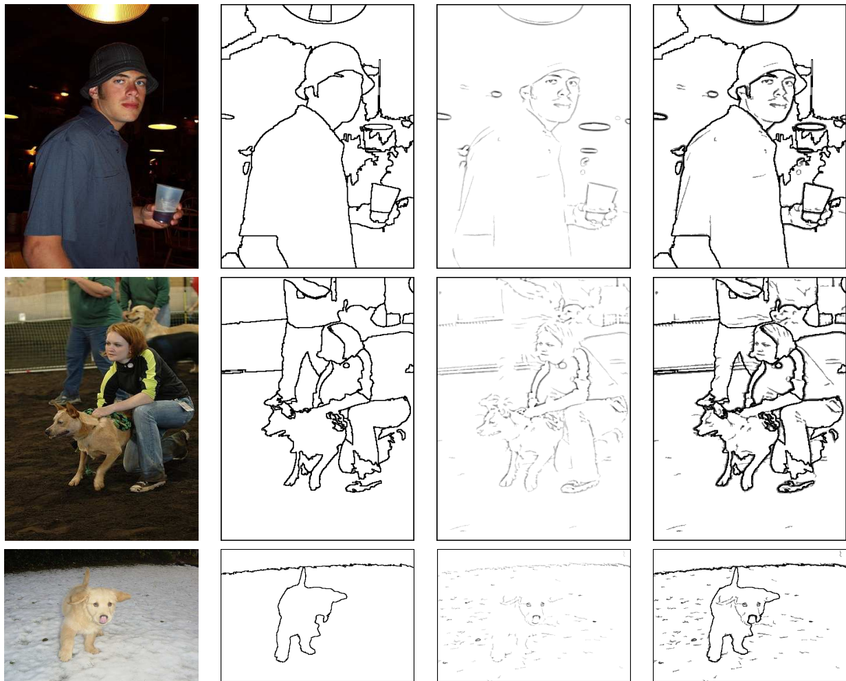
Figure 3: Example results for the system with addition of texture edges. In second column the results of the basic system B, in the third column the edge map obtained by the DoG algorithm normalized to [0, 1] and in the last column the weighted combination of them.
