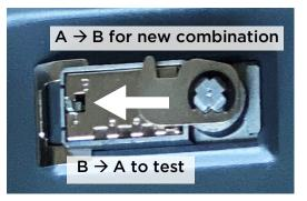
5. To test that the new code has been set, keep the safe open, turn the black knob on the front to the left. Change the numbers on the dial to a combination that is not the one you chose and see if you can turn the knob to the right. If you cannot turn the knob to the right, then you know that your new combination set. You may reset your combination as many times as you like.
