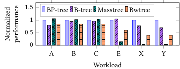
Figure 8: Relative performance compared to the BP-tree on uniform random workloads generated from YCSB.
