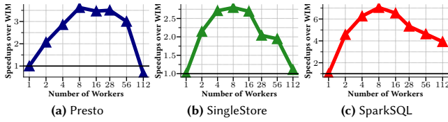
Figure 12: Varying the number of database worker instances on a dual-socket Intel Sapphire Rapids (geomean speedup with TPC-H SF 100)
